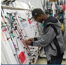
Top: MNSTAR employee tests a harness jig for a wiring harness that will be used by law enforcement
